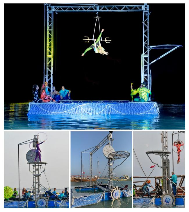
This is our pedal driven floating aerial platform. It provides all the elements of our land based Gantry Bike. While adjustable in size the standard size water device  $20' \times 20' \times 18'$  tall. Although its most unique feature is the rigging to support aerial acts, it also provides an elevated platform for ground-based acts. In the past to create this kind of effect, planners would need to build stages IN the pool. Aside from the steep cost of built in stage solutions
